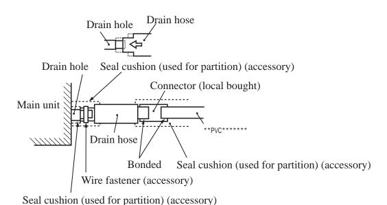
(d) When the equipped drain hose used to many units, the position of public pipe should be 100mm lower than the drain hole of any unit. As the figure shown. For this purpose, the thicker pipe should be used.
